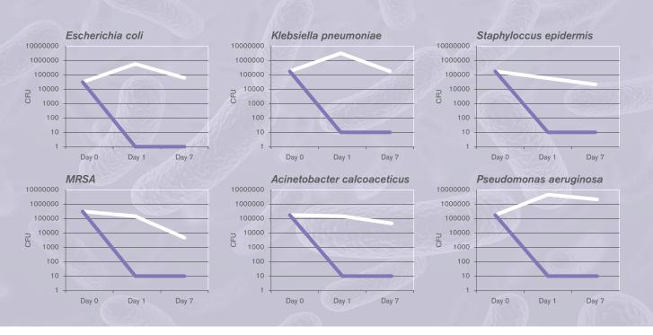
The addition of Silver Ion anti-microbial additive to Intersurgical breathing system tubing greatly reduces the viable microbial count level over time. The tubing has demonstrated a long lasting anti-microbial affect against a broad range of micro-organisms responsible for Hospital Acquired Infections. References: 1. Intersurgical Ltd. Certified Independent Test Results, 2003.
