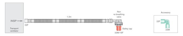
Code Description Box Qty. 2070000 22mm Flextube basic transport breathing system with non re-breathing valve, 12 for use with Oxylog® 1000, Pneupac® paraPAC®, ventiPAC™ and transPAC™, 1.2m
