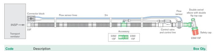
2072000 22mm Flextube™ transport breathing system, for use with Oxylog® 3000, 3000 plus and 2000 plus, 2m 10
