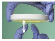
**5.** Check the smooth operation of the bi-directional anti-asphyxiation valve and place to one side.
